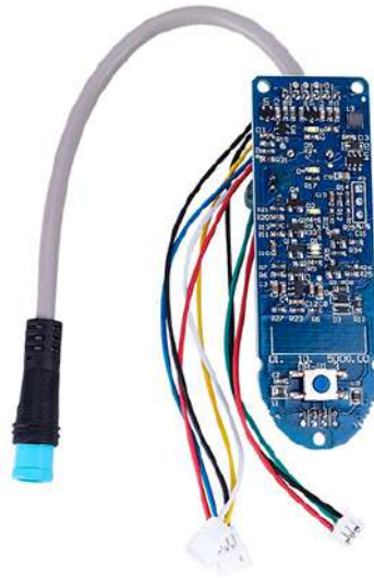
Figure 1.2. Xiaomi M365 BLE hardware components
